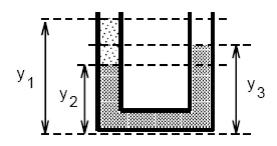
In the open manometer shown, water occupies a part of the left arm, from a height of  $y_1$  to a height of  $y_2$ . The remainder of the left arm, the bottom of the tube, and the right arm to a height of  $y_3$  are filled with mercury.
