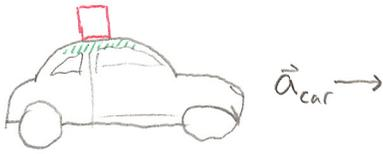
WITHOUT FRICTION, THE BOX WOULD SLIDE TO THE LEFT RELATIVE TO THE CAR ROOF. FRICTION ACTS IN THE OPPOSITE DIRECTION OF THAT RELATIVE MOTION. SO FRICTION ACTS TO THE RIGHT.
