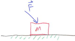
WITHOUT FRICTION, THE BOX WOULD SLIDE TO THE RIGHT RELATIVE TO THE FLOOR. FRICTION ACTS IN THE OPPOSITE DIRECTION OF THAT RELATIVE MOTION. SO FRICTION ACTS TO THE LEFT.
