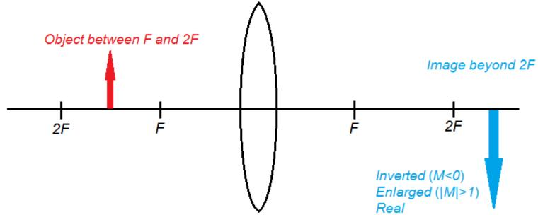
Slide projectors use this layout – the object is the slide; the enlarged image is projected on a screen.
