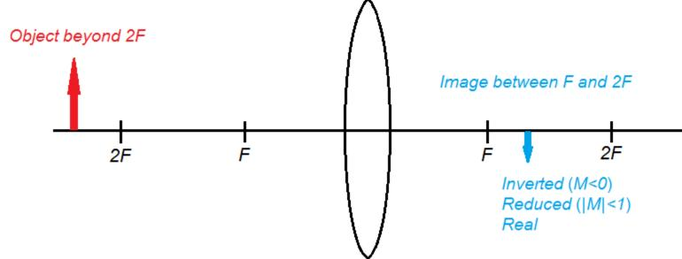
This is the arrangement of an eyeball lens or a camera lens; the eye's retina or the camera's film or CCD array is at the image position.
