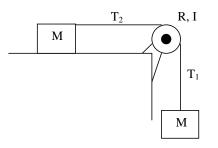
23. A falling block causes a disk to rotate. If R = 12 cm, M = 400 g, and m = 50 g, find the speed of m after it has descended 50 cm starting from rest. Solve the problem using energy-conservation principles.
