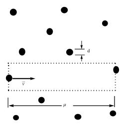
The mean free path  $\mu$  is the average distance a molecule travels in the gas between collisions. Suppose the molecules have diameter d. The moving molecule will collide with or hit a stationary molecule when the area of the moving molecule overlaps the area of one of the stationary molecules.
