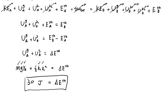
(c) A 2-kg box is compressed 1 meter against a spring whose spring constant is 20 N/m. Once released, the mass slides down a frictionless ramp then encounters a 1.0 m long section with no ice. The box comes to a rest at the end of the bottom surface. What is the coefficient of kinetic friction between the box and the bottom surface?
