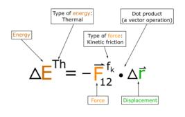
In words: The change in thermal energy of a system due to kinetic friction is equal to negative one times the dot product of kinetic friction between surfaces 1 and 2 and the displacement that the kinetic friction acts through.
