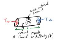
The above picture shows an object and the temperature difference, length, cross-sectional area, and thermal conductivity, k. The greater the distance the heat must flow, the slower the rate at which energy will transfer. With a greater cross-sectional area, there will be more atoms in contact and energy will flow more rapidly. Likewise, a larger temperature difference will provide a steeper "hill" resulting in a faster rate of conduction. Mathematically, this looks like the following:
