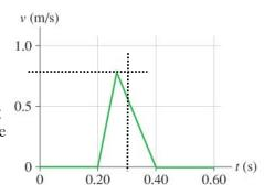
(a)  $a = \frac{\Delta v}{\Delta t}$  or slope of V(t)  $|a|_{\text{max}} \quad \text{between } 0.25 + 0.255$   $|a_{\text{max}}| \approx \frac{0.75 \%}{0.055} = 15 \% \text{s}$
