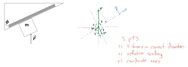
(b) Mass  $\mathbf{m}_1$  is a box which sits atop a frictionless incline of mass  $\mathbf{m}_2$  which sits on a frictionless surface. Do the analysis for both masses.
