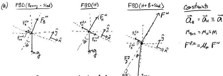
To find Friction forces, need Normal forces Fig. 12mg
