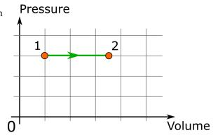
2. You have 2 moles of a monatomic gas that is initially at a temperature of 500 K. If 5000 J of heat is added to the gas, and the gas performs 7.5 kJ of work, what is the final temperature of the gas?
