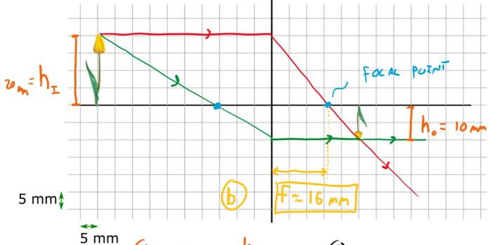
(a) Use a converging lens. A single diverging lens never creates a real image. A single converging lens can create a real image.
