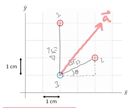
a)  $|\Delta \vec{r}_{13}| = 3cn = 0.63 \text{ m}$   $|\Delta \vec{r}_{23}| = \sqrt{2cn + 1c^2} = \sqrt{5cn}$  = 2.236cn = 0.022 m  $|\vec{F}_{13}| = K \frac{9.92}{|\Delta \vec{r}_{13}|^2} = 9.99 \text{ N}$   $|\vec{F}_{23}| = K \frac{9.93}{|\Delta \vec{r}_{23}|^2} = 17.98 \text{ N}$
