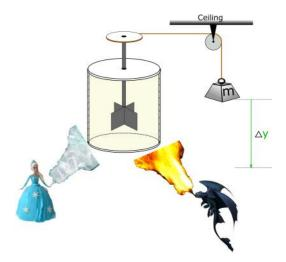
(b) A paddle wheel frictionally adds thermal energy to 5.0 moles of an ideal monatomic gas in a sealed closed container. The pad dle wheel is driven by a cord connected to a falling 2.0 kg mass falling shown in the figure. It is discovered that the temperature increased by 8 K doing the same 32 meter drop. Calculate the energy transferred via heat. Include the proper sign if the gas is the system.
