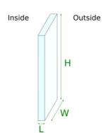
(b) The glass pane in a window has dimensions of 2.0 m by 1.5 m and is 4.0 mm thick. How much energy is lost in one hour? Ignore radiation effects and assume the glass has a thermal conductivity of  $0.78 \, \text{J/(m·s·K)}$
